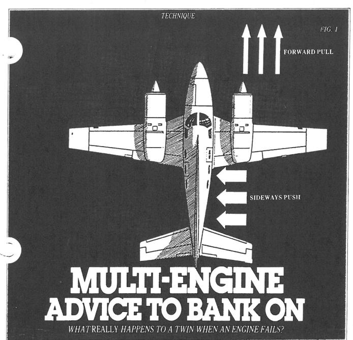
PILOTS OF multi-engine aircraft who suddenly experience an engine failure recognize the urgent need to maintain directional control. But many do not realize that, if the wings are held level and the slip/skid ball is centred during certain critical phases of engine-out flight, they unwittingly contribute to the loss of directional control. This may seem incongruous to those trained to maintain a wings-level attitude following engine failure. Nevertheless, it is true.
