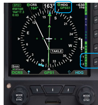
Figure 6-9 Operating in GPSS Mode
