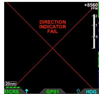
Figure 4-86 Direction Indicator Fail
