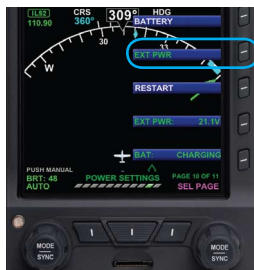
Figure 6-3 External Power Voltage Status
