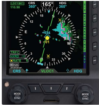
Figure 4-114 Horizontal Situation Indicator Showing Hazard Awareness
